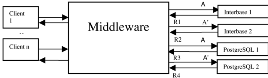
Fig. 2. A possible design for a fault-tolerant server using diverse SQL servers and data diversity. The original query ( A ) is sent to the pair {Interbase 1, PostgreSQL 1}, the re-phrased query ( A' ) is sent to the pair {Interbase 2, PostgreSQL 2}. The middleware compares/votes the results in one of the ways described in Section 3.2 for solutions without data diversity.
